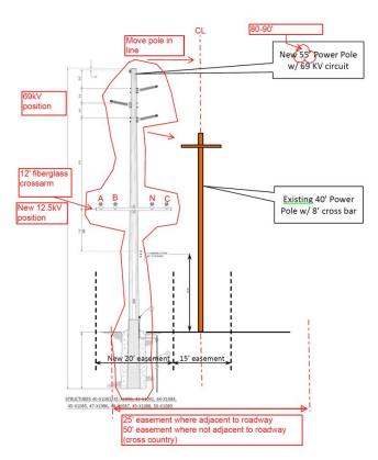
because UniSource must place the new poles in between the live electric circuits so as not to disrupt power to its customers. The advantage of the in-line, or "hot build," option is that UniSource can simply lift the existing 12.5 KV line onto the new under-build cross bar, saving over 36 miles of line (3 wires x 12 miles) which does not have to be spooled, transported and installed at another location in their service area.
